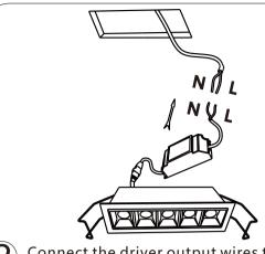
Connect the driver output wires to the main power( Please make sure the "L "and "N" to be connected in the right way)
