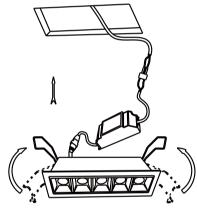
Put the driver into ceiling hole and push the clips into ceiling and make sure the fixture is fixed firmly
